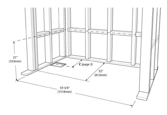
2A. Cut subfloor to accommodate plumbing in compliance with local plumbing and building code
