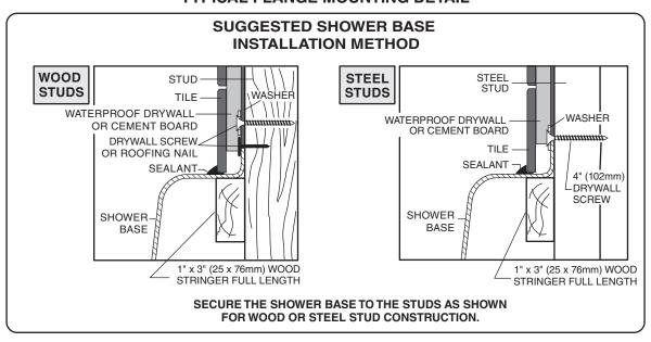
**C.)** Any finish material such as tile or wallboard must be self-supporting if it contacts the deck of the shower base. Flooring will be butted against the bottom of the shower base apron, also holding the shower base in place.
