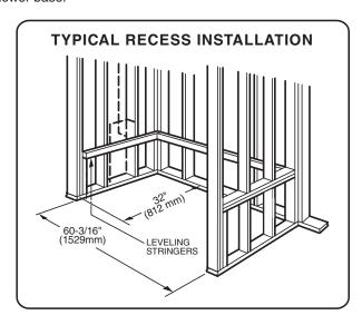
**B.)** Check level front to back and side to side, shim as necessary. To secure the shower base to wood studs, use drywall screws with flatwashers or roofing nails immediately above the flange of the shower base. To secure the shower base to steel studs, use 4" drywall screws and flatwashers.
